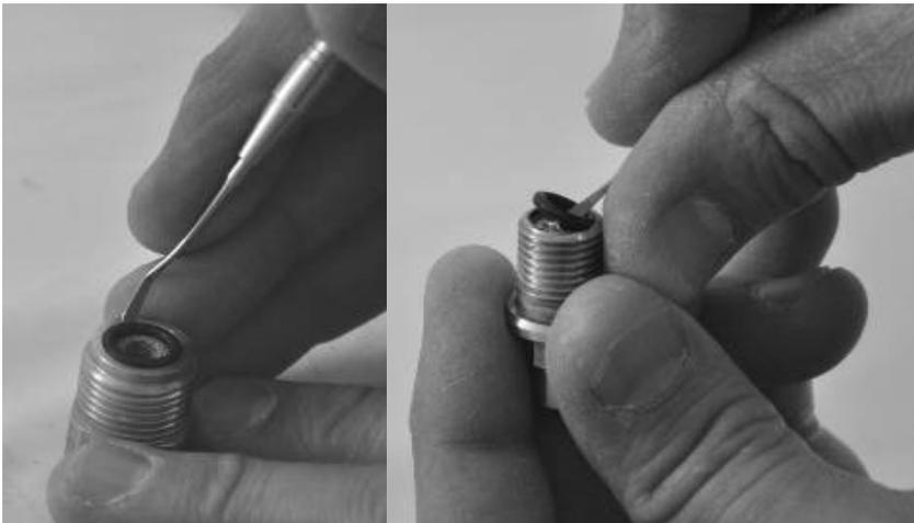
f. Remova o O-ring (444243) do parafuso DIN.
