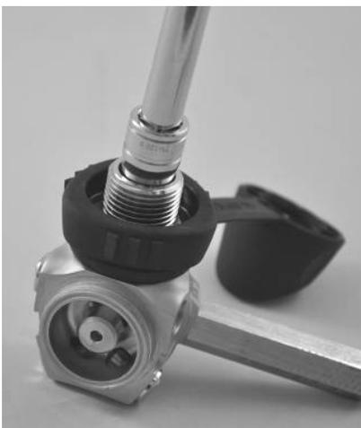
c. Remova o parafuso DIN (129213), o parafuso manual (129619/129722) e a tampa (129608).
